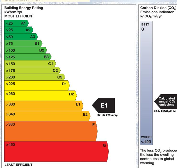
**Emissions Indicator** Calculated annual CO2 emissions 82.17 kgCO<sub>2</sub>/m<sup>2</sup>/yr The less CO<sub>2</sub> produced,
